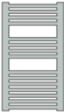
S45/75H Height 750 mm Width 450 mm Centres 410 mm Output 225 watts HE & E 150 watts
