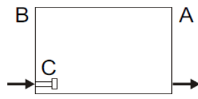
BOE bottom opposite end, side, left hand flow
