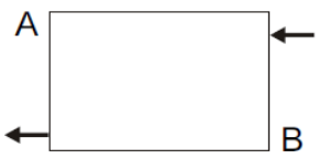
TBOE top-bottom opposite end, side, right hand flow
