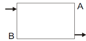
TBOE top-bottom opposite end, side, left hand flow
